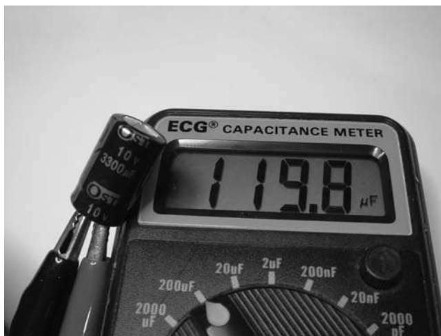
FIGURE 7-2 Bulging electrolytic capacitor with greatly reduced capacitance
