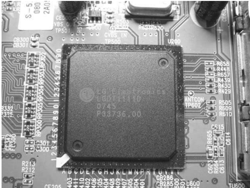
FIGURE 14-4 LSI chip with BGA contacts underneath
