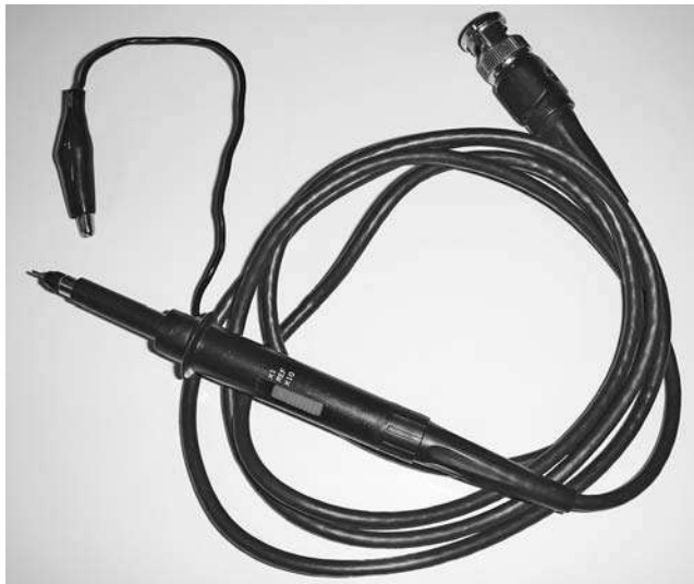
FIGURE 2-4 Oscilloscope probe, 10X/1X switchable
