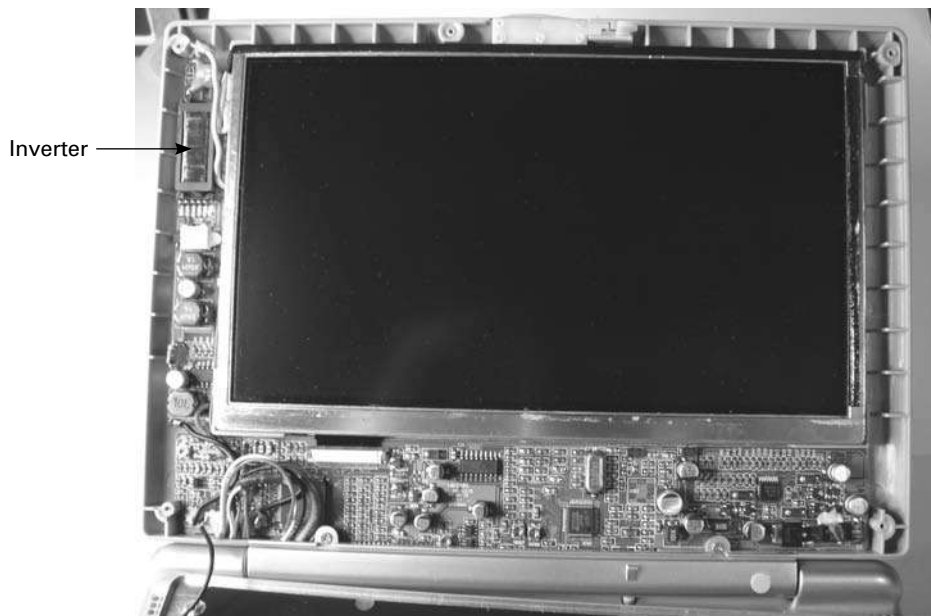
FIGURE 9-4 LCD with bezel off
